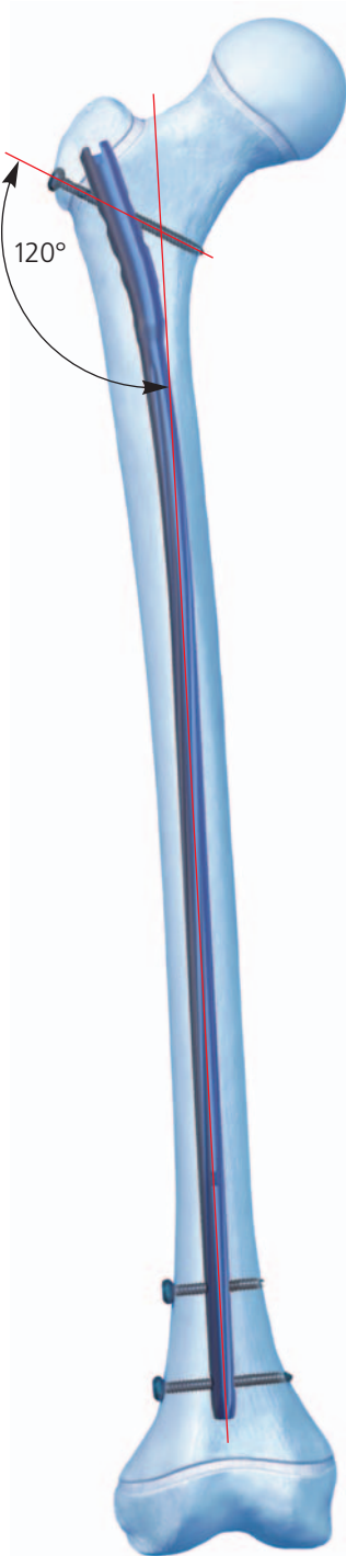
Proximal locking with 120° locking screw
