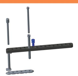
For optimal performance a closed frame shall be created with the plate. Drive a threaded sleeve and tissue protector into the last hole of the plate. This way the holes on the carbon element and those of the plate are aligned. Fix the carbon element firmly and check accuracy by placing a tissue protector and a threaded sleeve into any of the holes. They shall point directly to the center of the hole on the plate.
